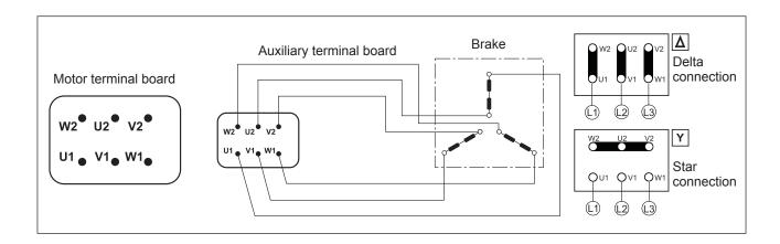
Wire the brake according to voltage and type of connection as shown on motor name plate.
