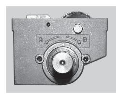
1. Drive the gearmotor until either one of the two end positions is reached. Disconnect power. While performing this, observe which direction the shaft is rotating, whether (**A**) or (**B**). Refer to raised arrows on side of the housing.
