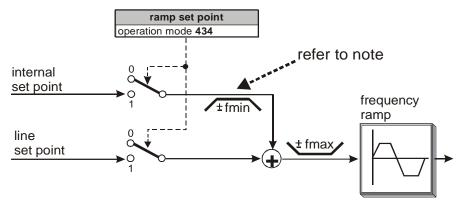
The internal reference value from the reference frequency channel and the reference line value can be led to the ramp individually or as an added variable. The operation mode of the ramp function is set via the data set switchable parameter *Reference ramp* **434**.
