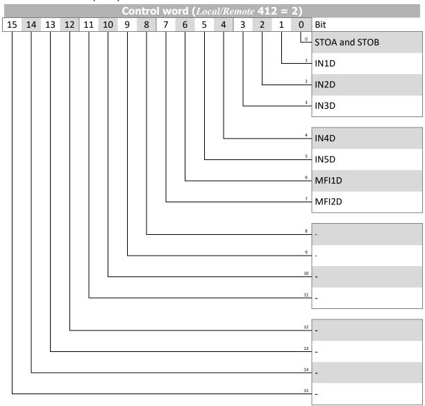
The digital inputs set via the control word can be monitored using parameter *Digital Inputs* **250**. Digital input STOA and STOB will only be displayed if controller release is switched on at STOA and STOB **and** the control word (Bit 0) was set. If the data set switching function is used, please ensure that Parameter *Local/Remote* **412** is set to "2 – Control via remote contacts" is set in all data sets used.
