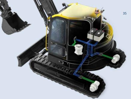
These two new products allow our customers to create a complete electrical solution for track and rotation drives dedicated to mini-excavators for the range from 2 to 4.5 tons. We are thus able to offer a completely electric alternative to the conventional axial piston engine hydraulic unit, reducing noise levels and consumption, as well as virtually zero CO2 emissions.
