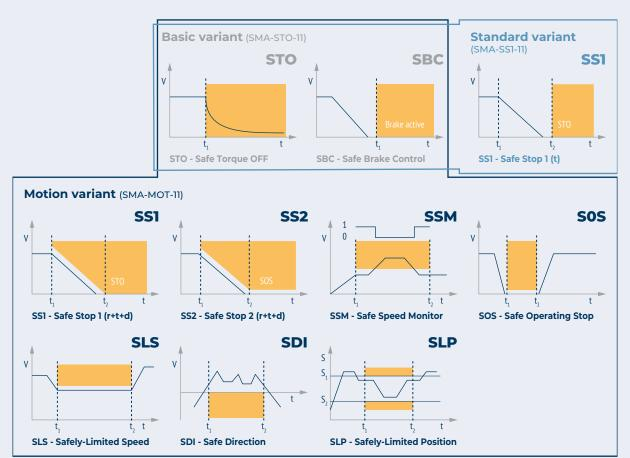
The Basic variant (SMA-STO-11) includes Safe Torque Off (STO) and Safe Brake Control (SBC), while the Standard variant (SMA-SS1-11) introduces also SS1-t (Safe Stop 1 with time monitoring) reducing the necessity for an external Functional Safety switch.
