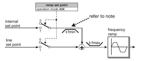
The internal reference value from the reference frequency channel and the reference line value can be fed to the ramp individually or as an added variable. The operation mode of the ramp function is set via the data set switchable parameter *Ramp set-point* **434**.
