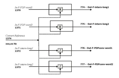
The standardization for In-F-PDP-word1/2 and Out-F-PDPconv-word1/2 is:
