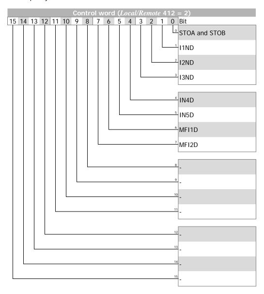
The digital inputs set via the control word can be monitored using parameter Digital inputs **250**. Digital input STO will only be displayed if controller release is switched on at STOA and STOB **and** the control word (Bit 0) was set. If the data set switching function is used, please ensure that Parameter Local/Remote **412** is set to "2 – Control via remote contacts" is set in all data sets used.
